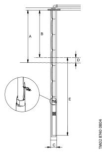
Fig. 10 Installation depth
