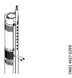
Fig. 8 Fitting the cable guard to the pump suction strainer
