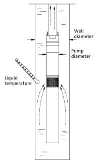
Fig. 1 Pump installed in well
