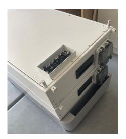
Dial correct addresses on modules (1-8 with 1 being at the top and 8 being at the bottom)
