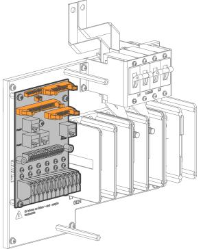
Carefully remove the four (12) M3 screws located at the top of the MPPTs terminals, then remove the remaining screws on the communications board.
