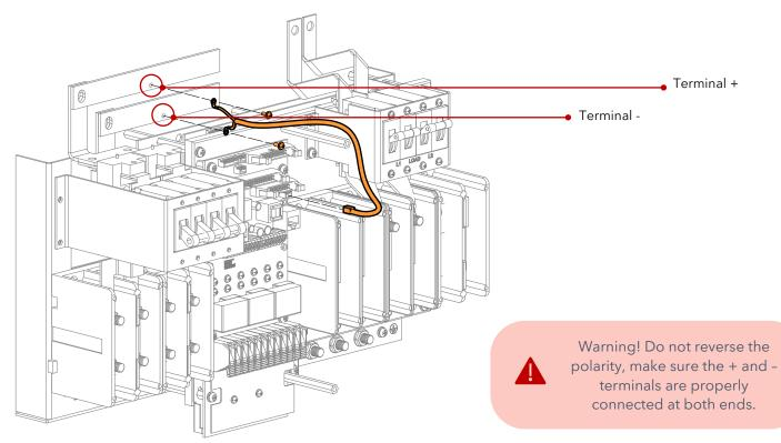
Connect the power cable to the "43-63V" input of the TX 15K-A board. Finally, reconnect the three (3) ribbon cables and three (3) connectors to the TX 15K-A board.
