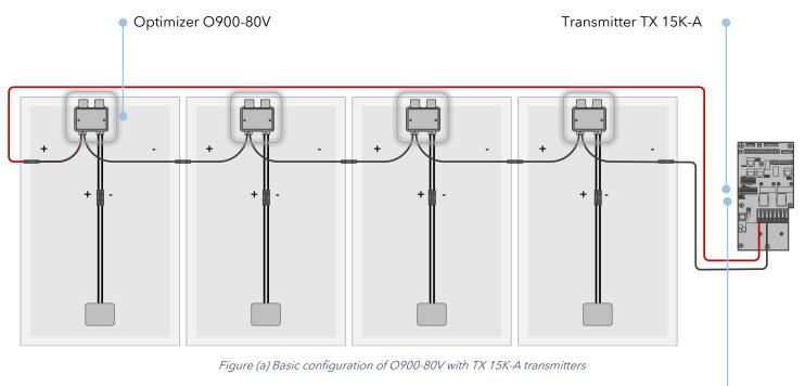
TX 15K-A mounts inside the Sol-Ark 15K-2P-N inverter
