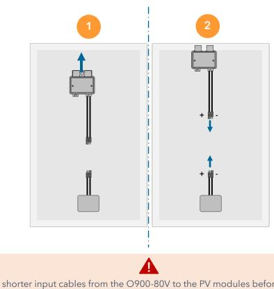
You must connect the shorter input cables from the O900-80V to the PV modules before connecting them to the string series with the remaining O900-80V. Failure to do so may damage the O900-80V units.
