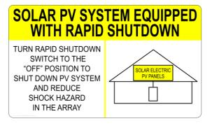
Figure (2.2) Rapid Shutdown System Label, NEC 690.12 (C)
