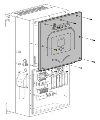
The top cover contains three (3) ribbon cables that power the LCD, you can slide the cover to the side of the inverter to avoid damaging the connectors.
