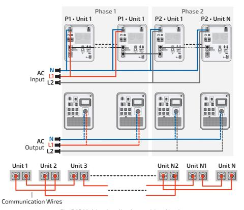
Fig. **5.16** Multi-unit split-phase wiring, N units
