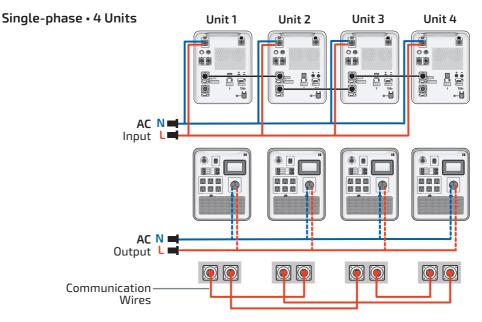
Fig. 5.12 Multi-unit single-phase wiring, 4 units
