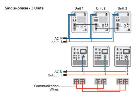
Fig. 5.11 Multi-unit single-phase wiring, 3 units
