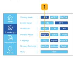
Select the Single P. button to set the unit's single-phase configuration (Fig. 6.22).
