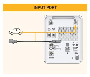
Fig. **5.6** Single unit - 120V DC input port and cable
