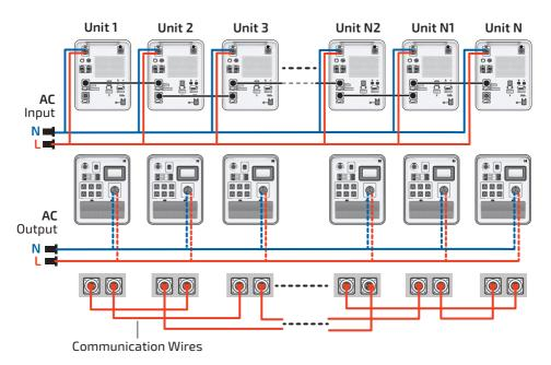
Fig. **5.14** Multi-unit single-phase wiring, 6+ units (N≤12)
