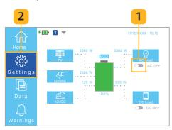
Fig. 6.15 Turn AC output switch OFF
