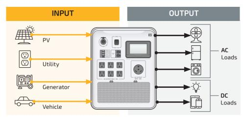
Fig. 5.3 Power options and output capabilities
