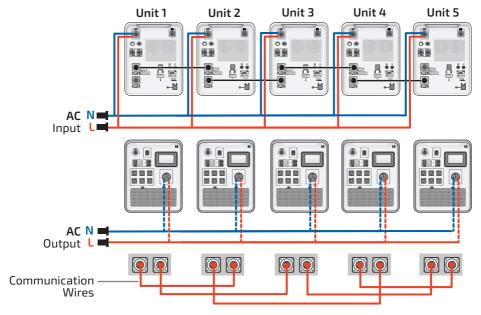
Fig. 5.13 Multi-unit single-phase wiring, 5 units
