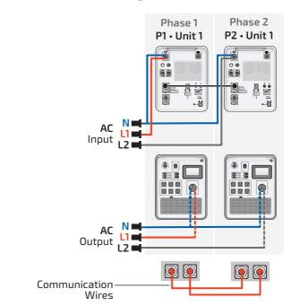
Fig. **5.15** Multi-unit split-phase wiring, 2 units
