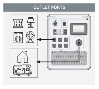
Fig. **5.5** 120V AC output ports
