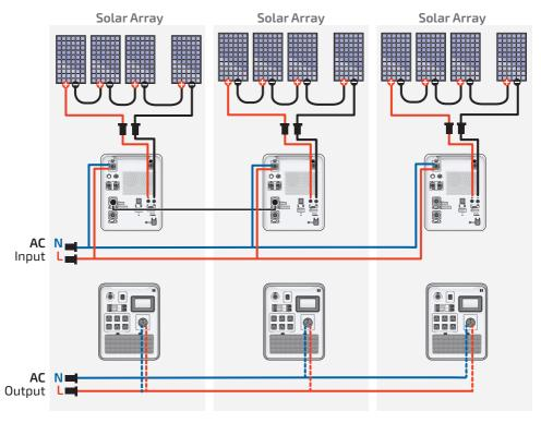
Fig. **5.19** PV (solar) wiring diagram for single-phase multi-unit systems
