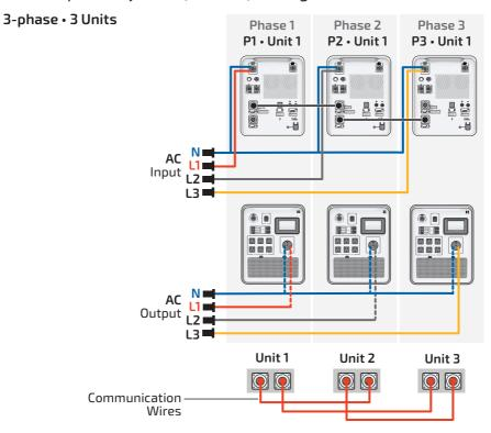
Fig. **5.17** Multi-unit 3-phase wiring, 3 units
