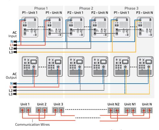
Fig. **5.18** Multi-unit 3-phase wiring, N units  $(N \le 12)$
