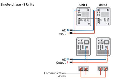
Fig. 5.10 Multi-unit single-phase wiring, 2 units
